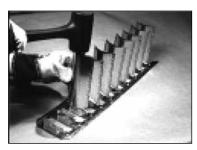
4. Insert the top rail tabs into the vanes.
